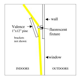
The valence should be placed so that most of the light shines up on the ceiling, and so that the bulb is not visible directly except from directly below the fixture. The back side should be painted white. Brackets can be made of 1x8 or 1x10 pine and placed between the four foot long fluorescent fixtures.
